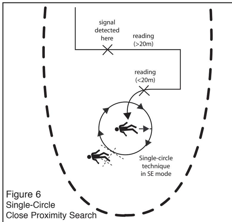
Remember that distance readings will always be greater for a vertically buried transmitter than for a horizontal one, even if they are buried the same distance from the searcher. For this reason, it is always important to maintain a tight circle; a victim with a vertically oriented transmit antenna may be closer than their distance reading indicates.
