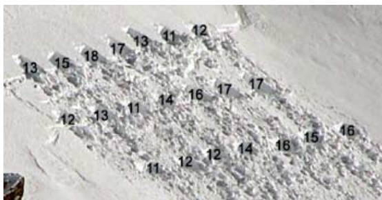
Figure 10: The ECTI scores from the 21 pits in Figure 9.
