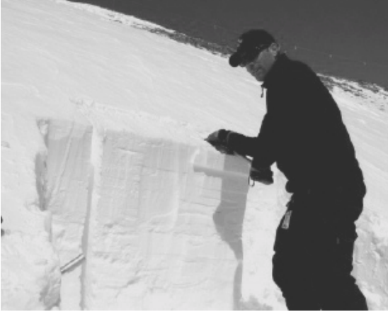
Figure 2: Example of a fracture that initiated but didn't propagate beyond the boundary of the loading area (shovel).
