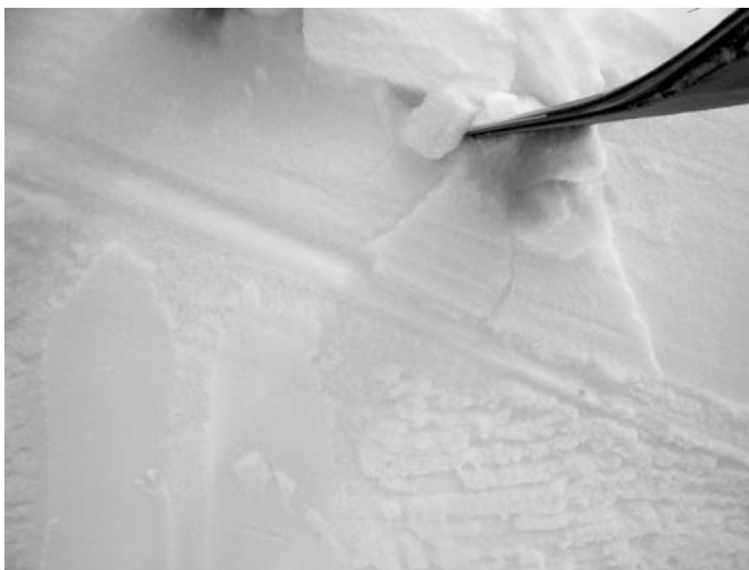
Photo 3: This is an example of excavated tracks from a ski cut where the skier did initiate a weak layer fracture beneath their skis, but the fracture didn’t propagate to release an avalanche. In this case the propagation propensity would be low, even though triggering was easy.
