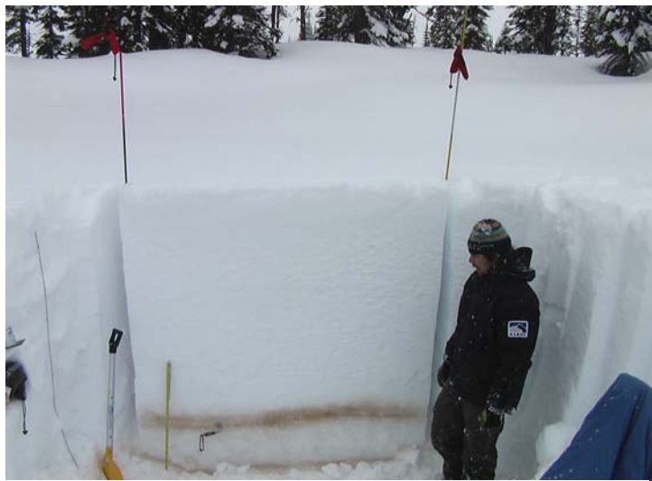
Photo 2: The slab we tested here was over 150 cm thick, and results from testing on this flat terrain were almost perfectly reproducible on nearby slopes. The PST works with slabs of any thickness, but columns like these can 30-45 minutes to prepare. The 3 m thick ones take hours.
