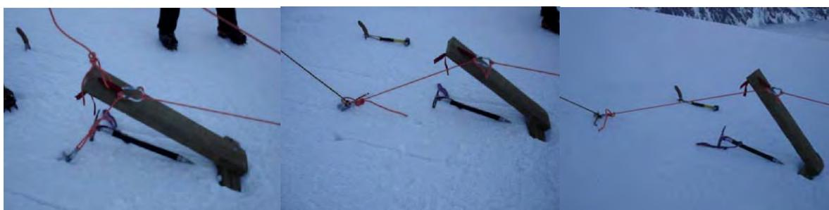
*Simulated belayer in the system. From left to right. 0.0 m, 0.5 m, 1.0m back from belay point. All photos were taken at point of failure*
