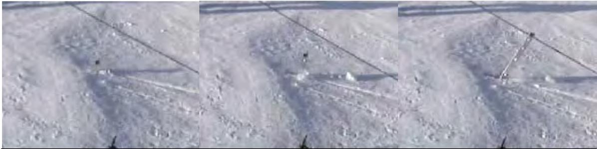
*This series of photos of an upright mid clip in at 10° back from perpendicular to the snow surface shows it lifting from the snow at around 3 kN. A similar sized stake set back 45° pulled down into the snow and failed at around 7 kN when the stake folded in the middle and the wire cable pulled out of it. The snow was cold <-10° C and between pencil and 1 finger in hardness. It was not possible to compress it to make stronger snow.*
