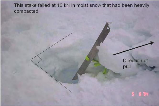
Observations of stress cone failures such as the photograph to the left in snow that has been manually compressed do not show clean shears of the entire cone. Weaknesses obviously exist inside the compacted snow, which mean that the actual shear surface is less than the theoretical area and therefore the strength will also be weaker than the maximum theoretical strength. However failures under shear are still relatively strong when compared to anchors failing under compression.
