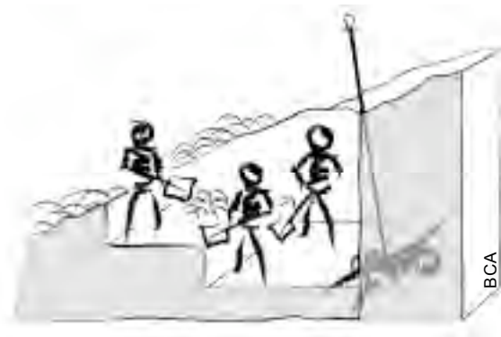
Figure 5. In burials deeper than two meters, it can be difficult to clear snow from the hole. Instead, it should be lifted to the next terrace, where it is removed by a secondary shoveler.
