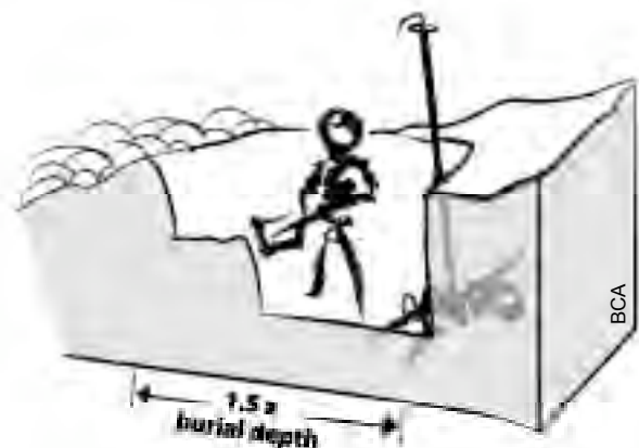
Figure 3. The optimal length of the hole should be 1.5 times the burial depth. Width should be 1.25 to 2 meters, depending on the number of shovelers.
